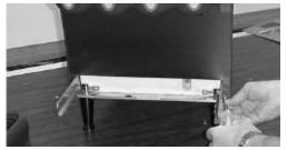
6. Slide the panel up and pull out to remove. On the 2 flavor unit it will be necessary to remove 2 screws from the back panel.
